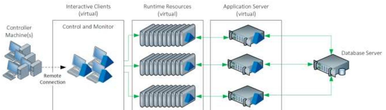
In the above example, each Application Server can marshal the connectivity for up to 100 Blue Prism Runtime Resources.
