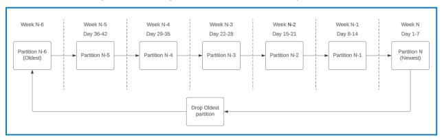
This solution requires a pre-planned database maintenance window to add, configure, and start the SQL Server partitioning (grouping) process. The Data Vault solution has little to no impact on performance, however Blue Prism Cloud will deploy and trigger the solution based on the Blue Prism Production Database's least busy time.
